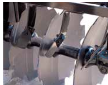
Tapered blades to improve leveling (2" front and 4" rear)
