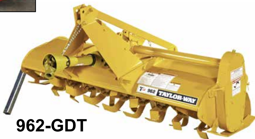
Tilling depth is controlled by adjustable skid shoes - to a maximum 8" depth.
