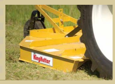
King Kutter's Heavy Duty Rotary Kutters are designed to meet the demands of today's farmer. This Kutter is built to perform. Durable, heavy-gauge 8" " I " beam side rails, and a fully reinforced 3/16" thick top-deck will stand up to tough conditions. HD gearboxes, slip clutches, and dual laminated tail wheels (6 ft & 7 ft models) are features that are standard on King Kutter Heavy Duty Kutters. The 7 ft HD Rotary Kutters are available as lift type.
