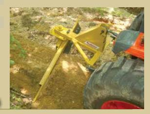
King Kutter's PRB Professional Rear Blades are designed for dependable performance on the tough jobs. The offset and tilt features, in conjunction with the industrial tube frame, make this a great blade for road ditch and driveway maintenance. The special formed moldboard and reinforced back bracing provide extra strength and performance.
