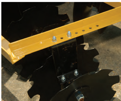
Bolt Style Gang Adjustment
