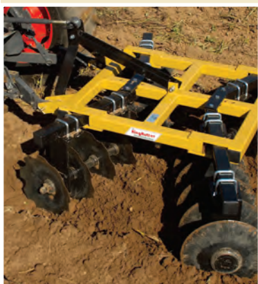
Box Frame Construction
